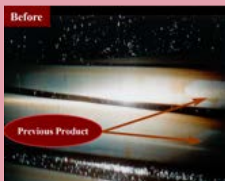
Lubricant film rupture evident. Lubricant did not meet OEM recommended viscosity for Open Gears.
