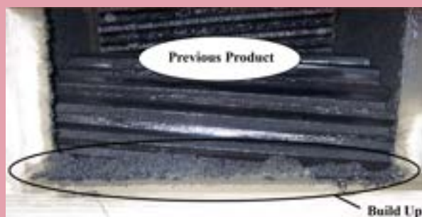
Lubricant build-up evident
