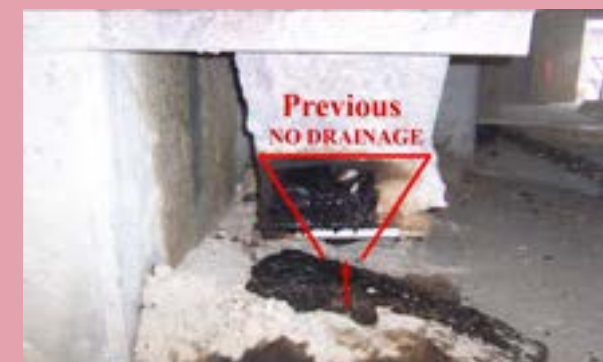
Drainage non-consistent / lacking proper drainage, build-up on gear guards, caused housekeeping issues.
