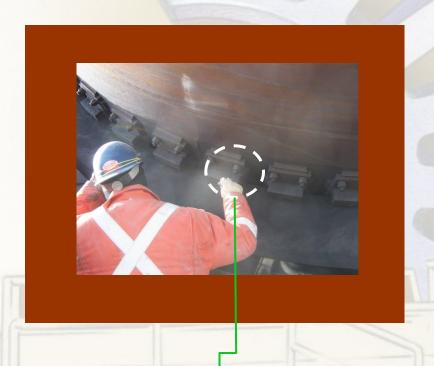
Easy Bar™ installed in tire slot every quarter turn (uphill rotation of kiln)
