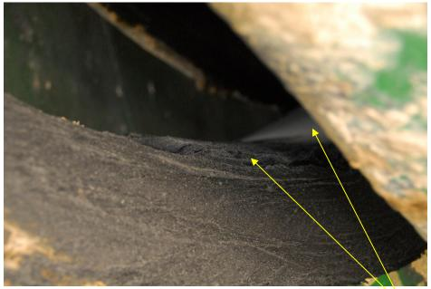
This is the transition area from loaded to unloaded. As you can see there is a grey matt appearance in the loaded area and the remainder of some previously added Walking cam lubricant has pooled up on the saddle in the noncontact zone.
