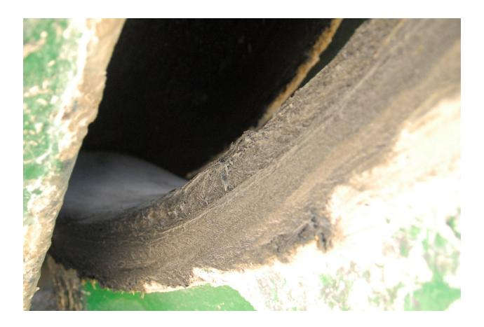
As you can see in the photo above there is good lubricant film coverage on the side of the saddle and no thin spots or base oil leakage.
