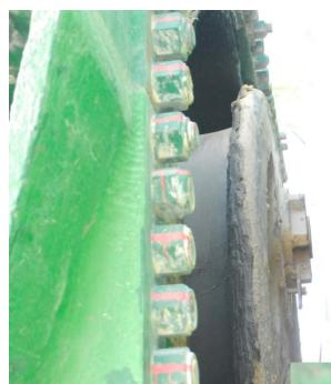
As seen in the next few photos the Walking Cam Lubricant is doing and exceptional job in protecting the cam with a heavy consistent lubricant film from edge to edge in the load zone. This dragline is 8 million pounds so each cam is lifting 4 million pounds.
