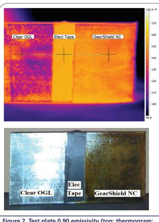
Figure 2. Test plate 0.90 emissivity (top: thermogram; bottom: photo). Clear OGL temperature: 132.4°F; Electrical tape temperature: 153.7°F; Gear Shield NC temperature: 150°F.
