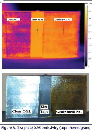
Figure 3. Test plate 0.95 emissivity (top: thermogram; bottom: photo). Clear OGL temperature: 130°F; Electrical tape temperature: 150°F; Gear Shield NC temperature: 146°F.
