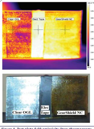
Figure 1. Test plate 0.60 emissivity (top: thermogram; bottom: photo). Clear OGL temperature: 150°F; Electrical tape temperature: 179.1°F; Gear Shield NC temperature: 173.6°F.
